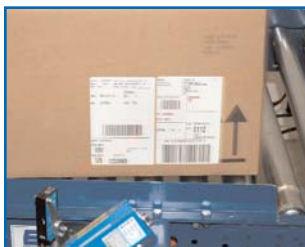
Barcode scanner checks label placement and detects any irregularities
