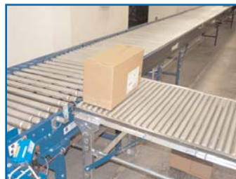
When problems are found, carton is sent down reject lane for manual inspection
