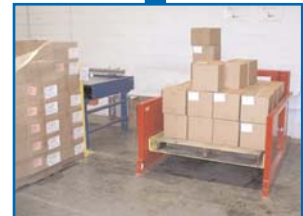
Ergonomic lift table accepts full pallets of product
